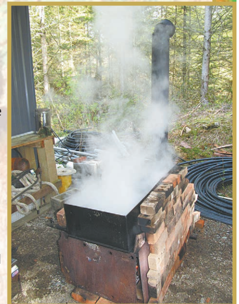
A stainless steel evaporator pan over a wood-fired arch.
