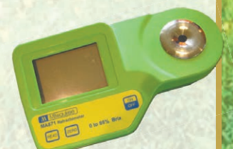
A refractometer measures the brix (sugar content) of a drop of liquid.
