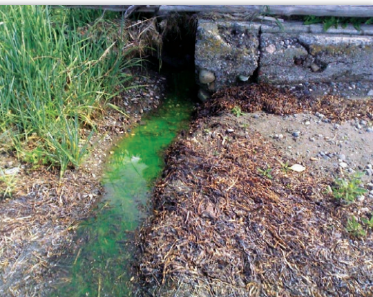
Above: A failed dye test in downtown Bay View – sewage was found to be flowing directly into Padilla Bay.
